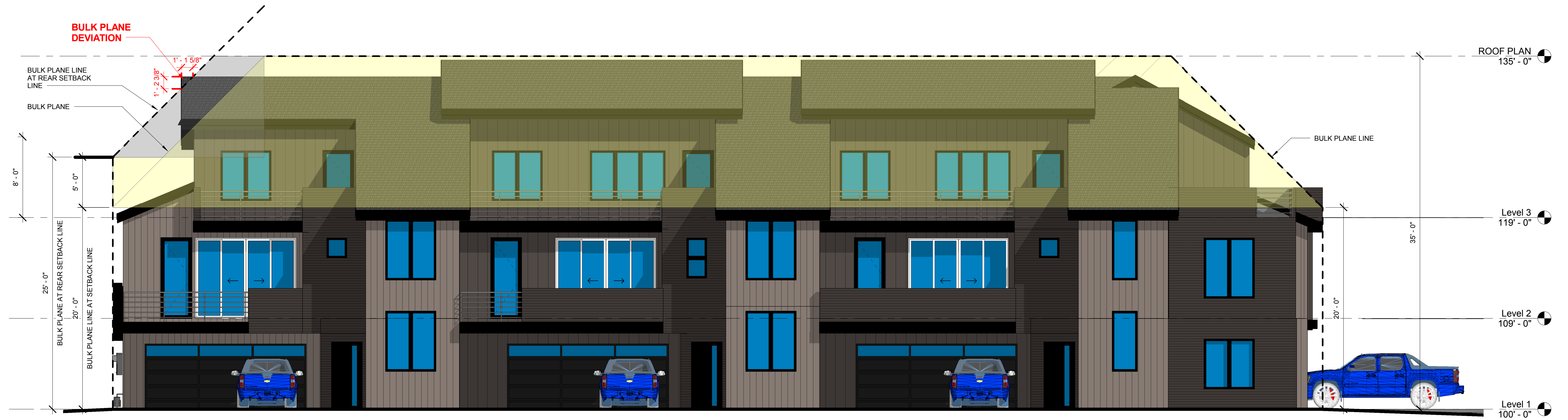
③ SOUTH ELEVATION BULK PLANE DEVIATION 3/16" = 1'-0"
