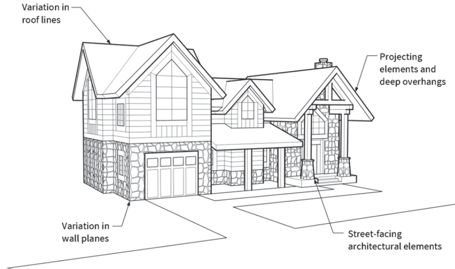
Figure 6-UU: Residential Building Design
