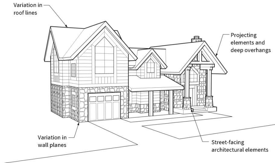
Figure 6-UU: Residential Building Design
