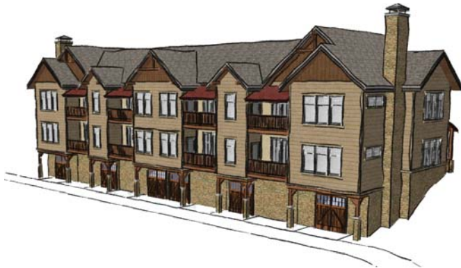
4.1 Tuck under garage parking at Townhomes
