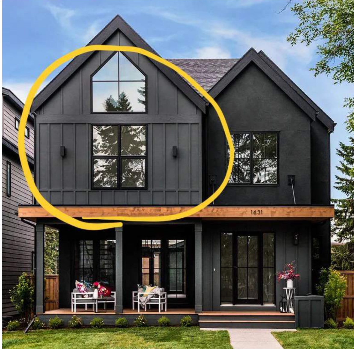
4. BOARD AND BATTEN (LARGE): 24" COMPOSITE BOARDS WITH 2X2 BATTENS 5. BOARD AND BATTEN (SMALL): 10" COMPOSITE BOARDS WITH 2X2 BATTENS 12. TRIM: COMPOSITE 2X2
